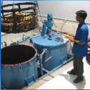
Vacuum Pressure Impregnation
