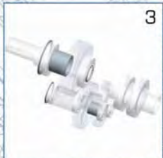
Mechanical parts locked in their positions by circlips and spacers. This also ensures better absorption of axial thrust and prolongs the life of bearings
