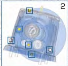
6 interchangeable plugs, including one breather plug and a level plug. Level and breather plug must be positioned according to this chart
